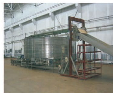
自堆积带式螺旋速冻装置 Self accumulation belt type spiral quick freezing device
